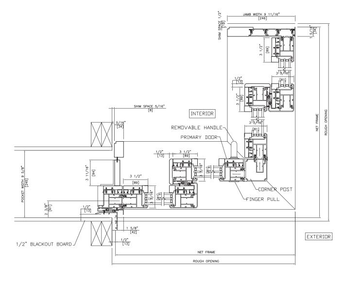
(90 DEGREE CORNER UNIT) STRAIGHT HEAD, RAISED THRESHOLD
