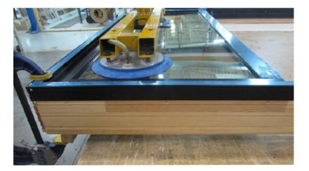
d. Pre-drill 7/64" holes through frame into panel along top, side and bottom. Pre-drilling 150mm from each corner and evenly spaced every 400mm.
