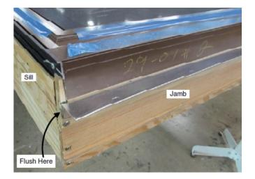
e. Apply a 5mm bead of Bostik Pro MS50 sealant (#49819) in X pattern on side flange, as shown below, where head flange will overlap.
