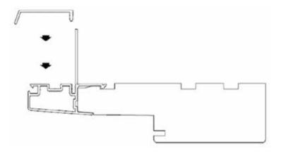
2. Apply drip cap onto frame cladding.
