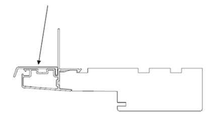
**Note:** Drip cap should be centered on head and equal OSM width, with a tolerance of  $\pm .25$ mm.
