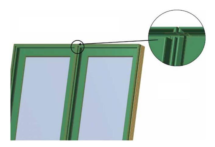
1. Where required, remove accessory kerf fins with a grinder to allow fins of mullion cover to run through. Refer to previous page.
